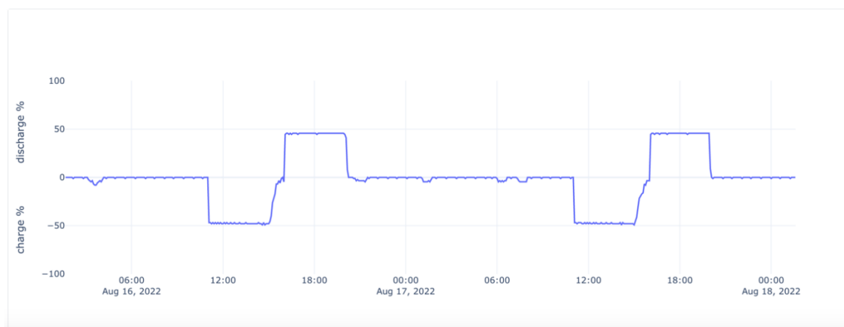
Figure 2.5: A snapshot of the daily charge/discharge ratio of the Fitzroy North community battery.
